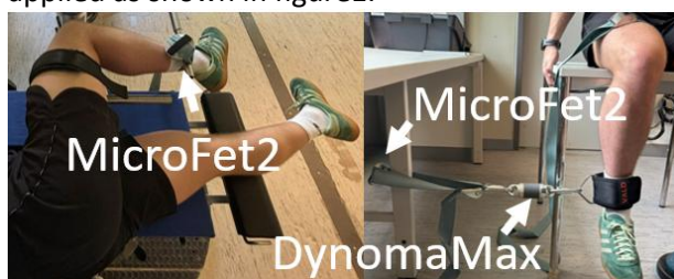
Fig. 1: Measurement of hip external rotation strength. Left: Side lying position in ISOMED2000 plus MicroFet2. Right: Sitting position with MicroFet2 fixed to table and DynamoMax.
