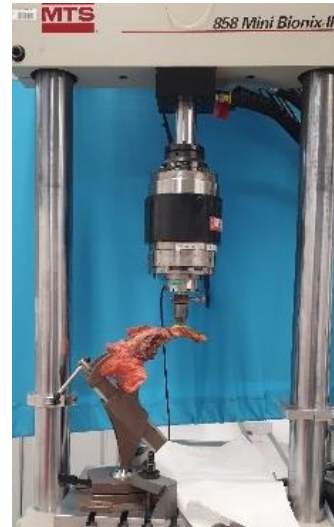
Fig. 2: Specimen mounted on the table of the material testing machine
